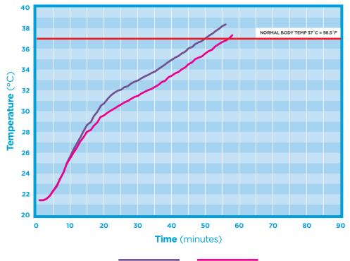
Samples are 4"X4"X4" 3.0lb/ft³ density, 10 IFD, 4 CFM Airflow and placed in a 104°F oven.
